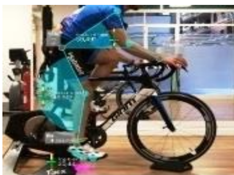
Figure 4. Knee flexion analysis with the crank at 180^\circ (Holmes, Pruitt & Whalen, 1994)
