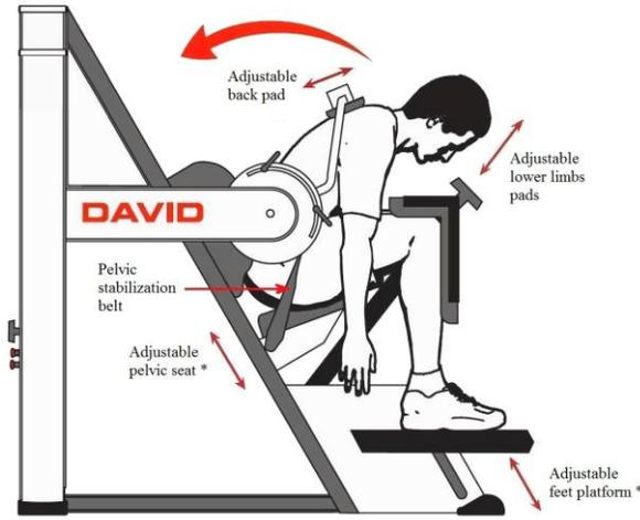
\* Feet and pelvic position is adjusted in raport with subject height, to get an angle of approximately 90 degrees between thighs and calves.
