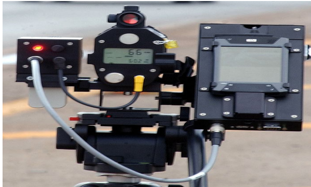
Fig 2 show Microdigicam Laserto measure shot speed
