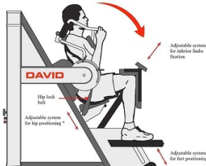
* Hip and feet position adjustment is accomplished according to subjects height, to obtain an angle of approximately 90 degrees between thigh and calf.
